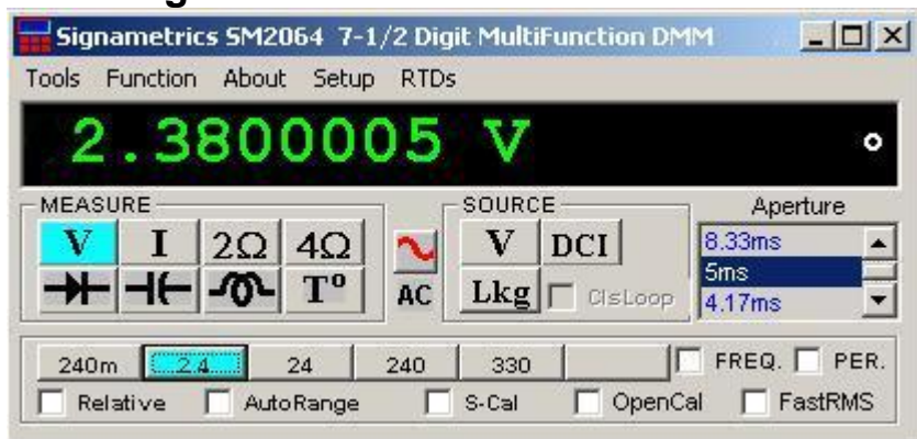
Figure 3-6. The Control Panel for the SMU2064. The three main groups include Measure, Source and Range buttons. The Range buttons are context sensitive such that only “240m, 2.4, 24, 240 and 330 appear when in AC Voltage Function is selected, and 2.4m, 24m, 240m and 2.4 appear when AC Current functions is selected, etc.
