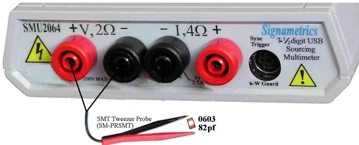
Figure 4-11. Measuring capacitors or inductors is best handled with low capacitance shielded probes.
