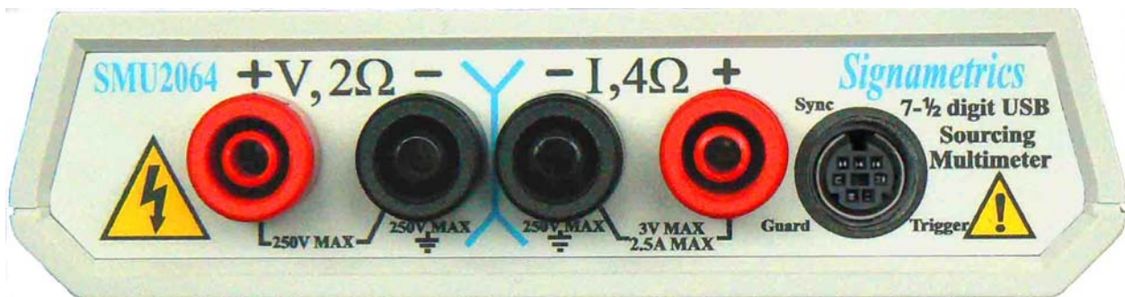
Figure 3-1. The DMM input terminals include both, four Banana and a DIN-7 connector.
