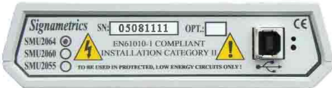
Figure 3-6. The Rear panel has the USB BF type connector. Compatible with BM cable.
